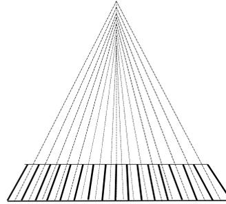
Figure 5. Variable focal length fan-beam collimator.
