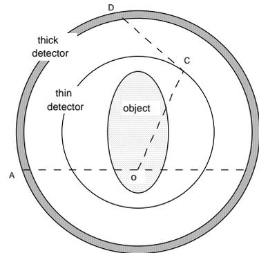
Figure 13. A double ring detector system for detection of triple photon emissions. The cone surface from the single photon detection and the line from the pair photon detection intersect at two points for the emission site.
