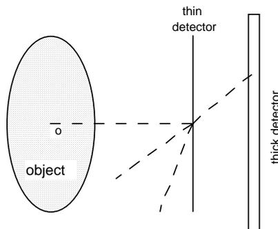
Figure 12. A photon emitted from point O in the object will be scatter (only once) by the thin detector and then detected by the thick detector. The two interaction sites determine a line. The energy deposited in the thin detector will give the scatter angle. So a cone surface is given with the line being its axis.
