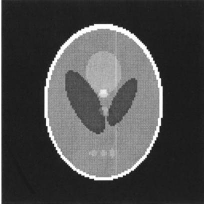
Fig. 5. The Shepp-Logan phantom by  $128 \times 128$  digitization. This phantom is the sum of the gray values of ten ellipses. Each projection of this phantom can be analytically computed.
