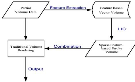
Figure 1. The flowchart of our feature-based rendering algorithm.
