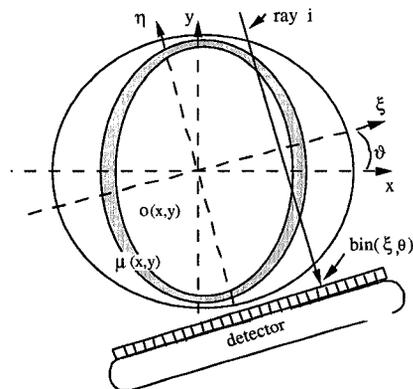
Figure 1. Data acquisition configuration for SPECT imaging. The  $z$ -axis is the rotation axis.
