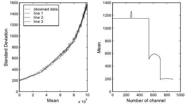
Figure 4. Left --- Standard deviation-mean curve and three fitting lines. Right --- Mean distribution of segmented transformed data.
