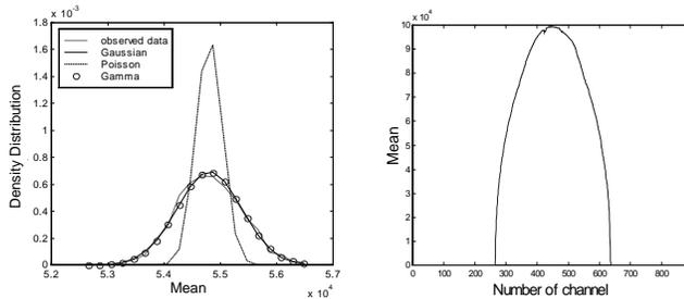
Figure 1. Noise property of acquired low-dose CT projection data. The number of channels per view is 888 and the number of measurements is 900. Left: PDFs of channel 600. Right: Mean distribution of the data across the channels.
