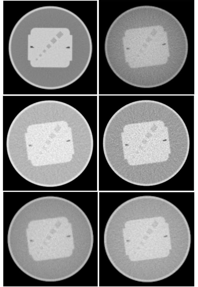
Figure 6. Comparison of reconstructed CT images using different filtering approaches. Top: left --- noise-free; and right --- noisy. Middle: left --- Hanning filter (cutoff frequency  $f_c = 0.25$ ); and right --- Hanning filter ( $f_c=0.40$ ). Bottom: left --- log transform + Wiener filter; and right --- segmented log transform + Wiener filter.
