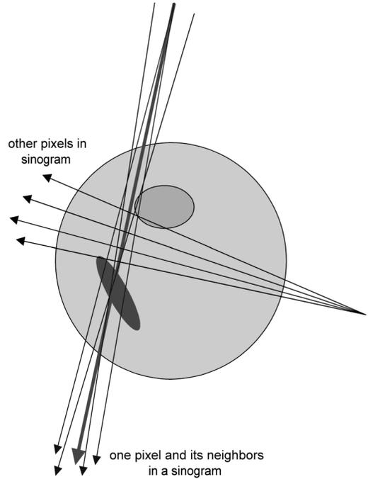
Fig. 2. Different property of a Sinogram from other piece-wise images. The intensity of one pixel in a sinogram is determined by the object being scanned, which can be estimated from the whole sinogram. Therefore, all rays, not only its neighbors, provide useful information.
