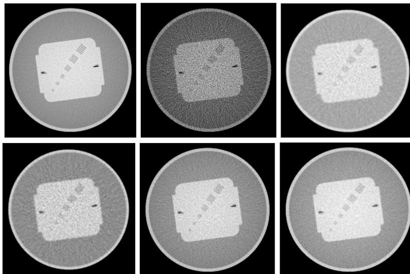
Figure 2: Comparison of FBP reconstructed CT images using different filtering approaches. Top from left to right: noise-free result, noisy data result with Ramp filter, Hanning Filter (cutoff frequency  $f_c$  is 0.25). Bottom from left to right: Hanning filter ( $f_c = 0.40$ ), K-L domain PWLS with  $pc$  (number of principal components) = 5,  $\beta = 5$ ; K-L domain PWLS with  $pc = 3$ ,  $\beta = 20$ .
