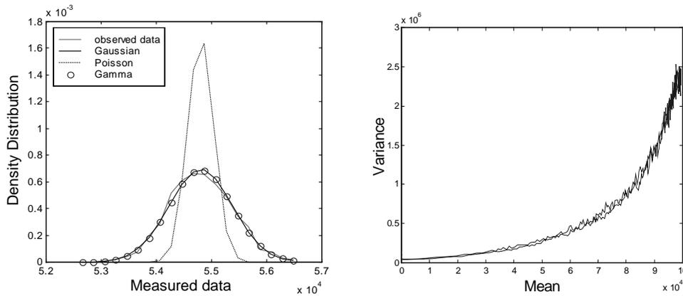
Figure 1: Noise property of acquired low-dose CT projection data. The number of channels per view is 888 and the number of measurements is 900. Left: PDFs of channel 600. Right: Variance-mean curve.
