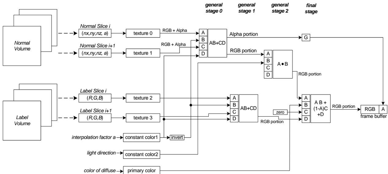
Figure 1: Register combiner setting for 3D reconstruction.
